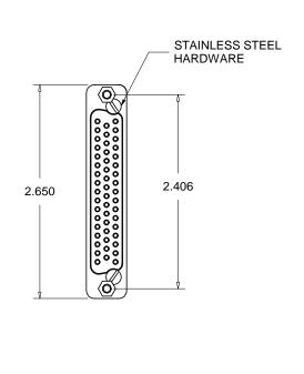
① - JACK SCREWS ARE REMOVABLE. DEPENDING ON THE TYPE OF MALE CONNECTOR USED, MODIFICATION TO THE JACK SCREW OR THE CONNECTOR MAY BE NECESSARY.
